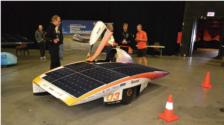
The winning car from Brunel/Delft University Solar Team, the rebuilt Nuna11S, which is a three-wheeler that weighs just 157 kg.
