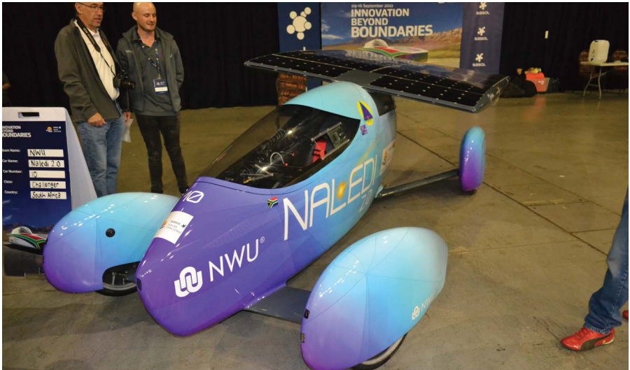
Naledi 2, the solar car from NWU weighs only 170 kg and features a unique rotating solar array.
