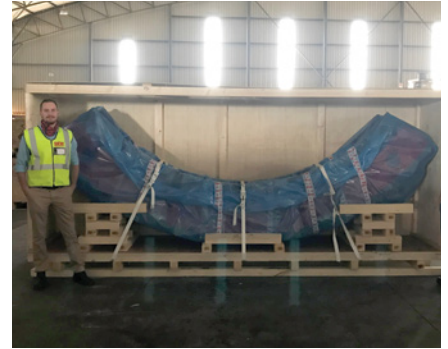
Left: SEW-EURODRIVE girth gears installed on the secondary scrubbers at De Beers Venetia Diamond Mine in Limpopo province. Right: The segmentation of girth gears makes for easier packaging, transportation and handling.
