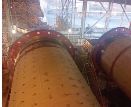
Left: SEW-EURODRIVE girth gears installed on the secondary scrubbers at De Beers Venetia Diamond Mine in Limpopo province. Right: The segmentation of girth gears makes for easier packaging, transportation and handling.
