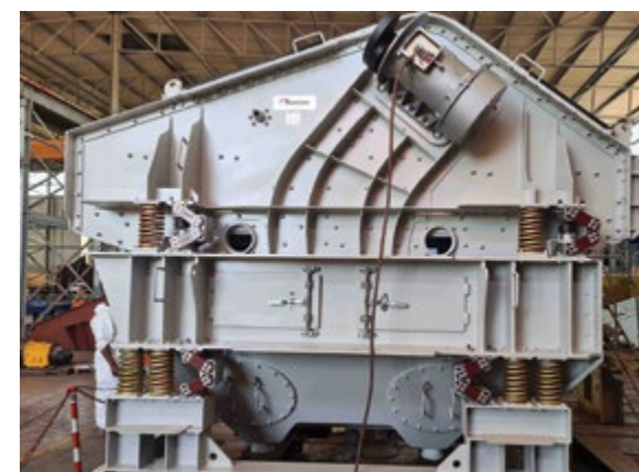
Left: A smaller Kwatani vibrating screen fitted with torsional springs for the diamond mining industry. Right: The fully adjustable test screen in the Kwatani laboratory for testing of dry commodities.
