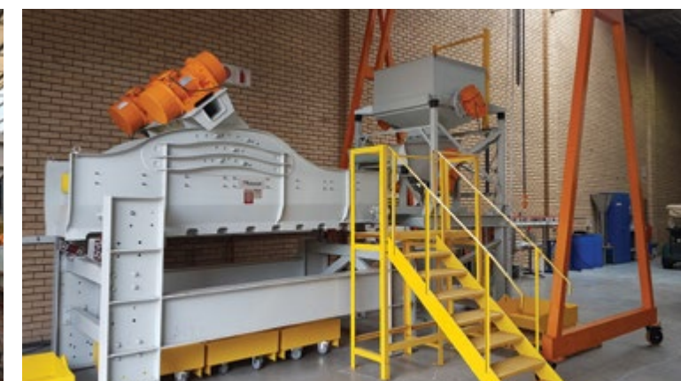
Left: A smaller Kwatani vibrating screen fitted with torsional springs for the diamond mining industry. Right: The fully adjustable test screen in the Kwatani laboratory for testing of dry commodities.
