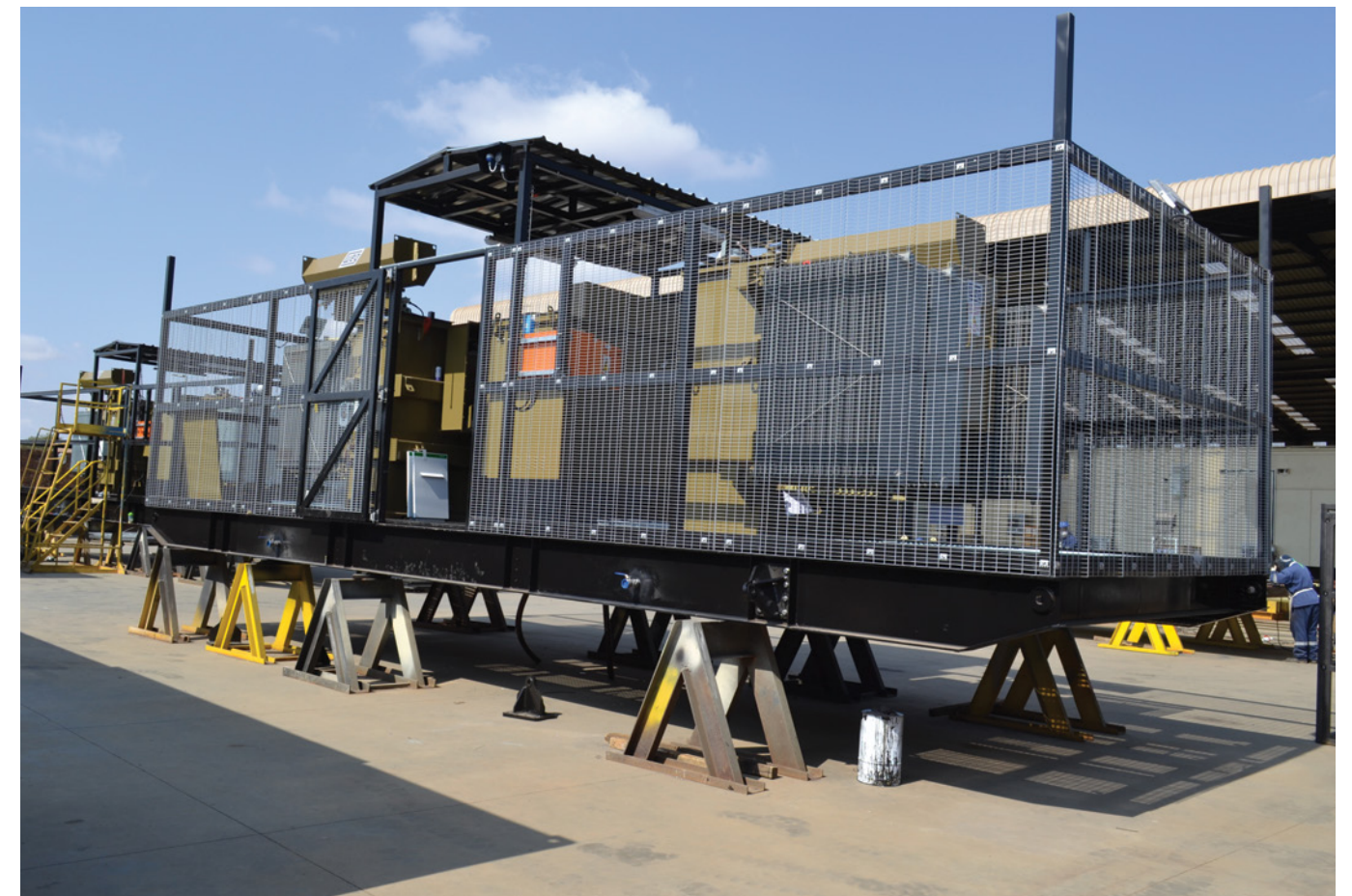
A skid-based transformer platform under construction at Zest WEG's E-House manufacturing facility in Heidelberg, South Africa.
