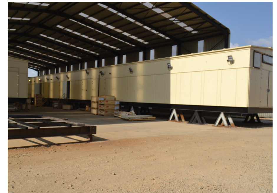
A three-roomed 45 m portable mini-substation with a 6x6 m cross sectional area destined for the hot environment of an iron ore mine in Northern Cape.
