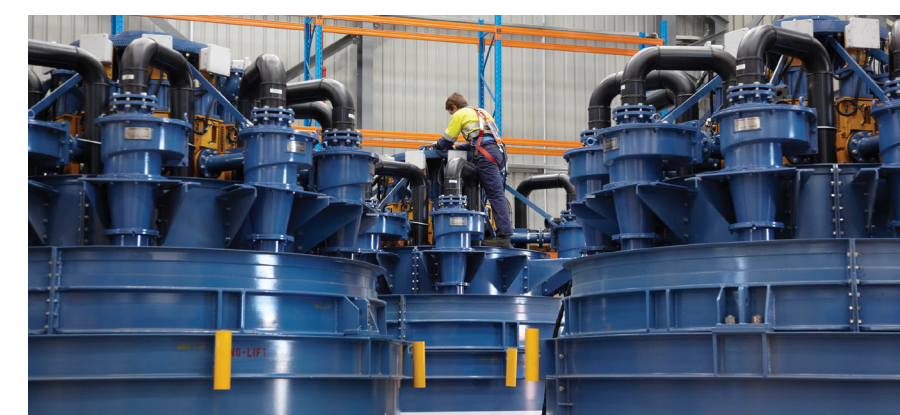
KREBS® cyclone manifolds have at least two cyclones on standby. As soon as roping or unstable discharge is detected, the operator will be informed via the SmartCyclone™ system and action can be taken.
