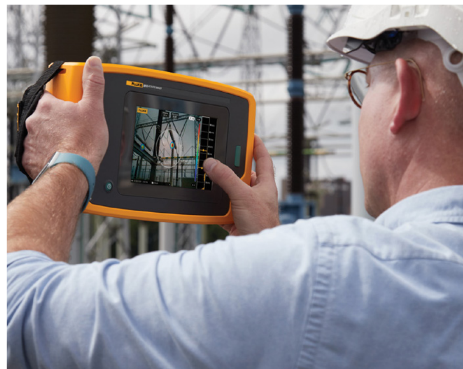
Fluke's ii910 Precision Acoustic Imager has dual uses: for the detection of compressed air leaks and particle discharge.
