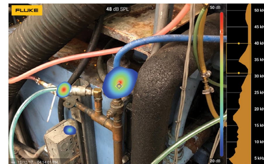
Fluke's ii900 Industrial Acoustic Imager captures still and video images of compressed air leaks at a facility.
