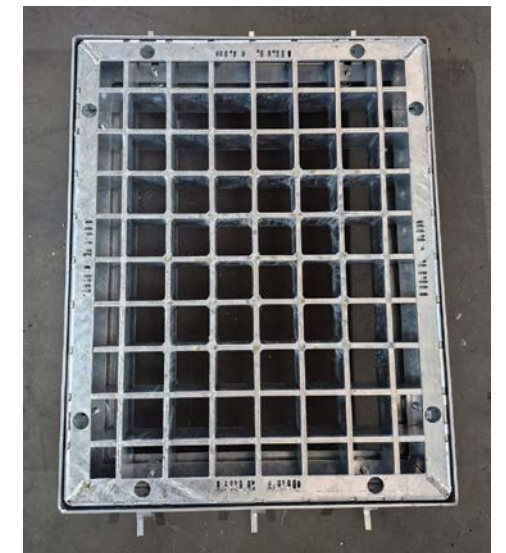
Jubilee Suppliers manufactures, under licence, a patented grid for storm water drainage. The bars are precision-cut with slots, assembled into a grid, and then welded at the end of each bar to secure the grid structure.
