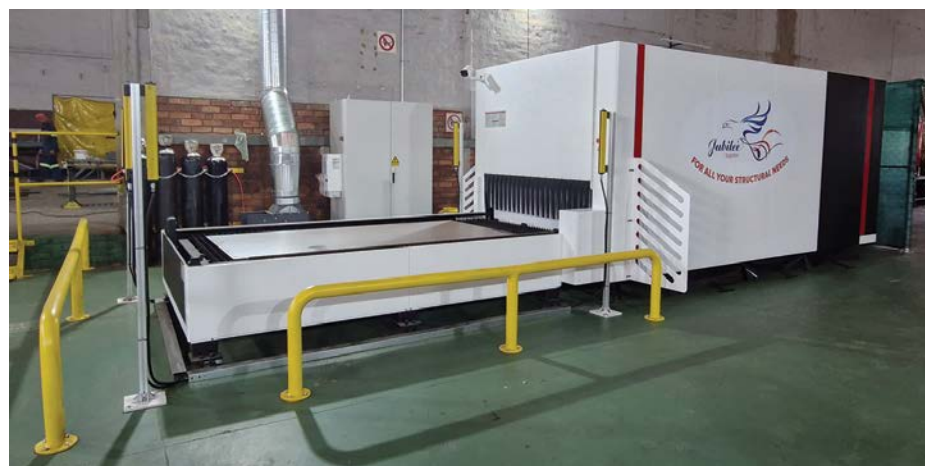
Jubilee Suppliers' new 6.0 kW Jinan Acme CNC cutting system, recently acquired from Cosmo Group, features a Max Photonics fibre-laser cutting head, a 3.0x1.5 m double-exchange worktable, and a fully enclosed laser-cutting area.
