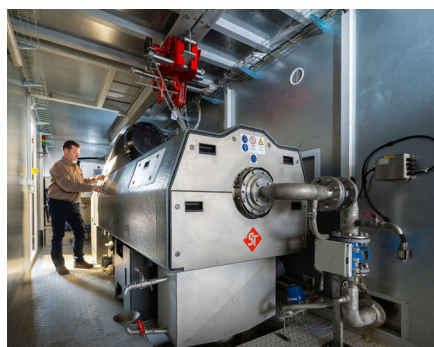
Left: The Multotec demonstration and decanter centrifuge comes in a 40-foot container with a small footprint.
