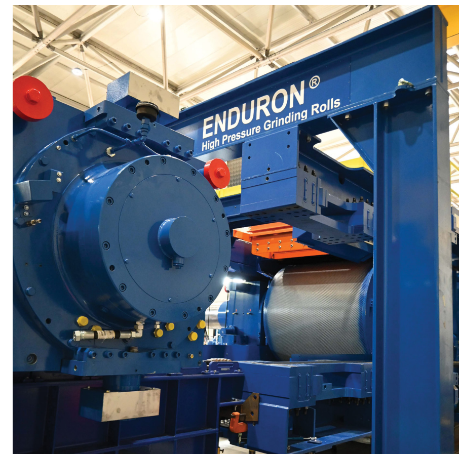
Mines are adopting HPGR circuits as an energy-efficient alternative to the traditional semi-autogenous grinding (SAG) mill circuits.
