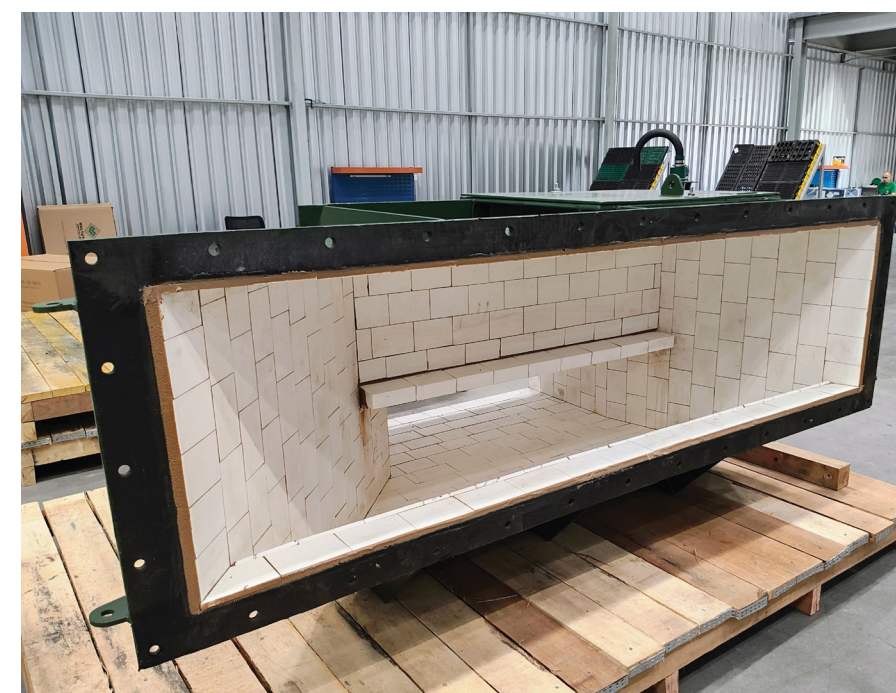
Left: Multotec lined 23 chutes in Brazil and will redesign and line new chutes using insights from current wear patterns to improve wear resistance. Right: A lithium producer in Brazil upgraded its chutes from rubber lining to Multotec's custom ceramic lining, achieving a significant improvement in wear life.
