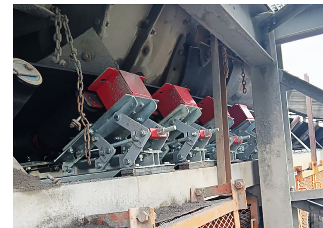
Left: The impact idlers in the Tru-Trac EXHD system oscillate to adjust dynamically to the load, significantly reducing the force transmitted to the belt. Right: Tru-Trac's EXHD dynamic impact idler bed represents a significant advancement in conveyor belt protection.
