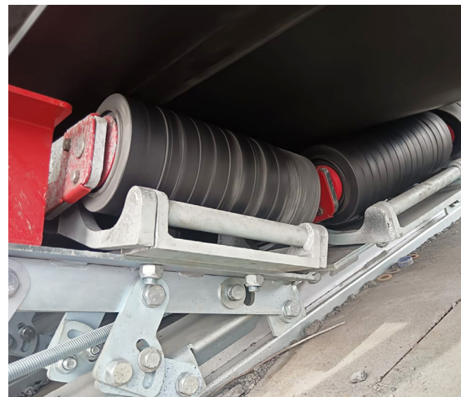
Left: Tru-Trac's EXHD dynamic impact idler bed provides a durable solution to protect belts and improve system reliability in demanding conditions. Right: The EXHD combines dynamically adjusting impact idlers with robust shock-absorbing springs to provide superior impact control.
