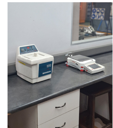
Some of the GFTC’s precision laboratory equipment: a Branson 1510 ultrasonic cleaner used to separate clay from sand grains in a sample, and an Ohaus Explorer precision balance for achieving an exact chemical composition of a melt.
