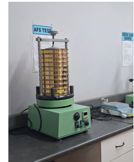
Left: The GFTC’s pattern-making shop: The college is introducing digitalisation, with employees moving from manual design to computer-aided design. Middle: A trainee doing sand preparation at the GFTC’s foundry using a green sand mixer. Right: A motorised sieve shaker for sand testing and quality control.
