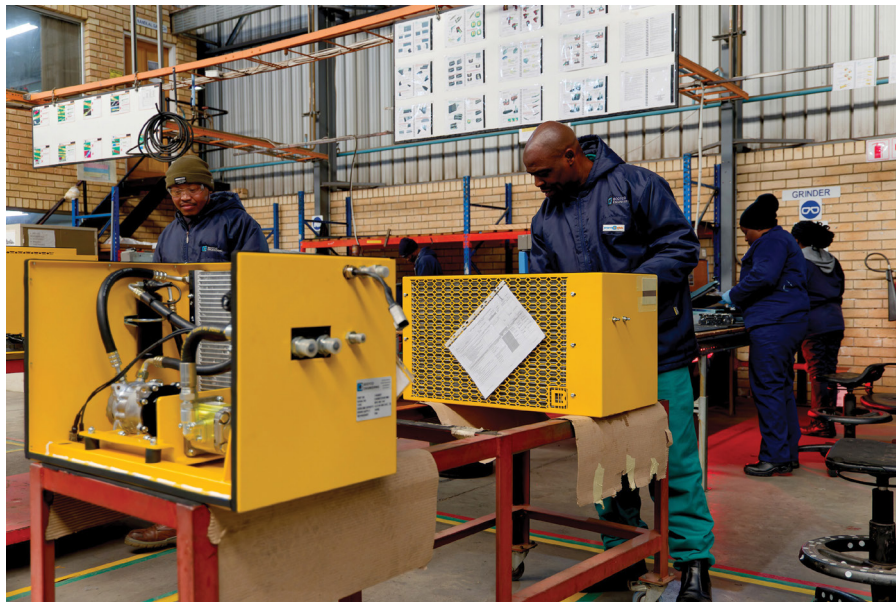
Engineered to meet ISO 23875 requirements, Booyco Engineering's cab climate control solutions ensure clean, pressurised air and effective CO 2 management for safer operator conditions.
