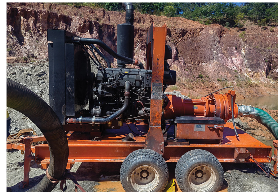
With Godwin diesel-driven units proven in remote and high-head applications, Integrated Pump Technology ensures that mines maintain reliable dewatering even when electrical supply is unstable or unavailable.
