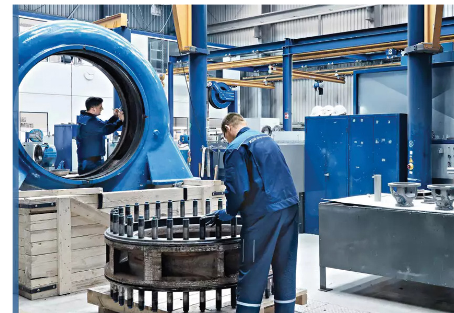
KSB's Jet Park Workshop comprises 4 400 m 2 of under-roof space, eight fully equipped work centres for refurbishing the KSB pump range, and three dedicated work centres for refurbishing boiler-water recirculating pumps used during boiler start-up or shutdown.
