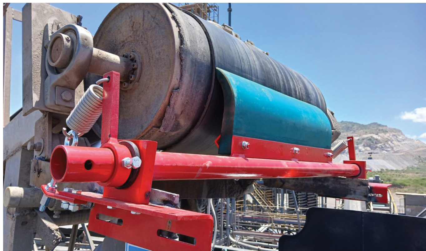
The primary cleaner on a conveyor belt sits on the drive pulley beneath the discharge stream and handles about 90% of carry-back material.
