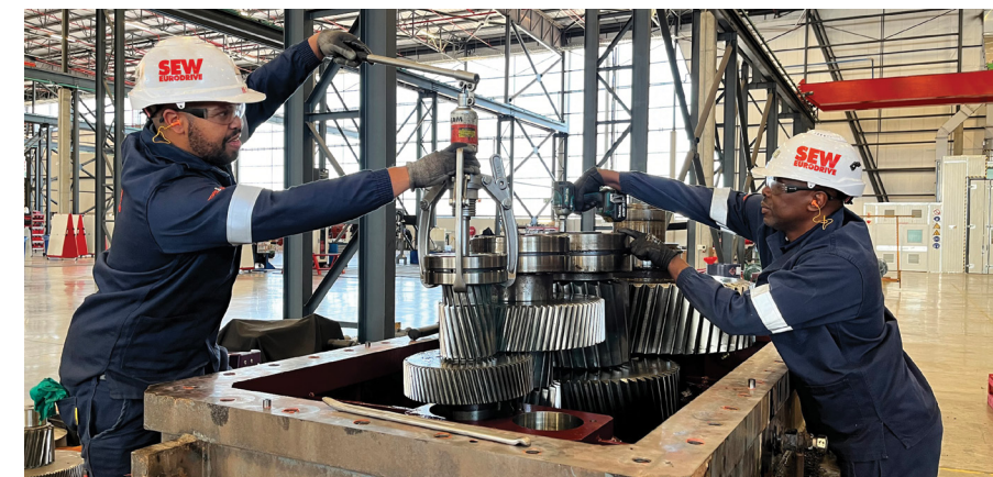
In the workshop, specialist technicians strip, assess, and rebuild gearboxes using high-precision processes identical to those used to assemble new SEW-EURODRIVE units.
