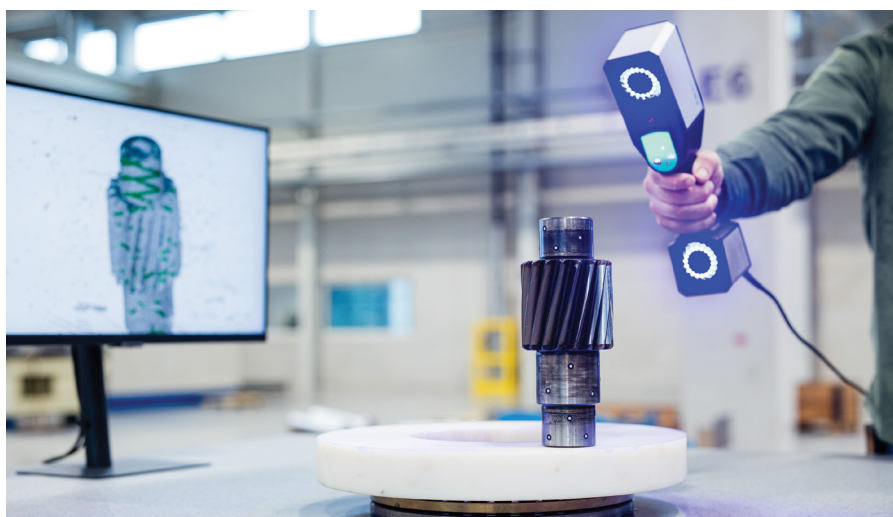
Laser scanning technology enables SEW-EURODRIVE to accurately map worn components and reverse-engineer complete gearsets to OEM specifications.
