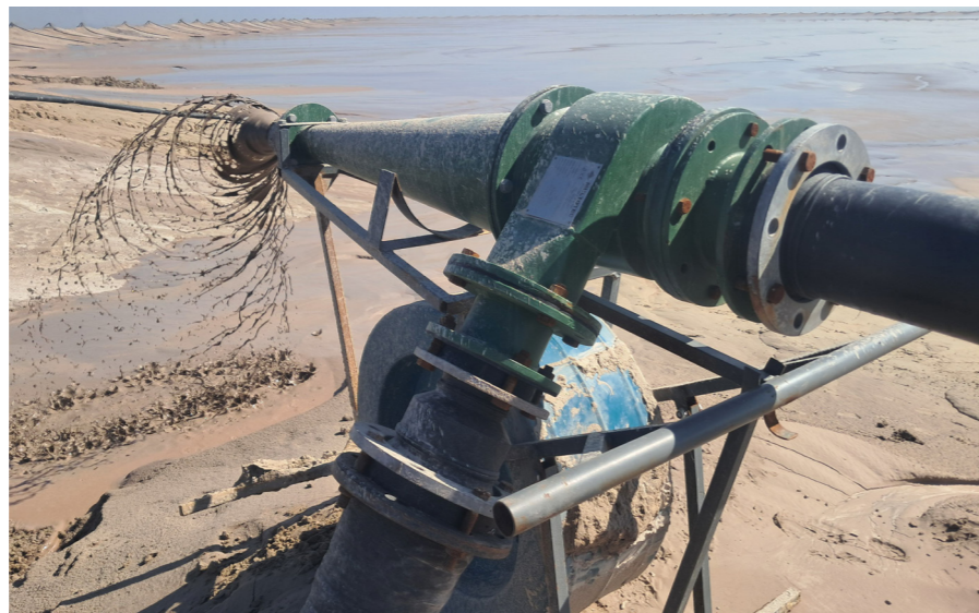
Their lightweight, durable design, simple spigot change system, and adaptable components make Multotec's GV Cyclones an operator-friendly and technically reliable solution for tailings dams.
