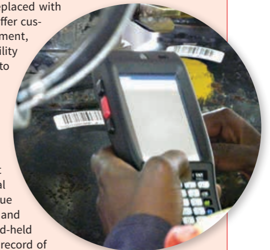
All Aprox industrial, special and medical gas cylinders now carry a unique barcode, which is scanned during delivery and collection using a state-of-the-art hand-held device to create an immediate electronic record of the transaction.
