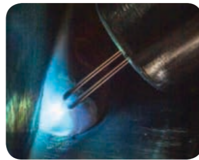
Unlike traditional multi-wire processes, which typically require dual power sources or dual contact tips, HyperFill uses a single power source, wire feeder, welding torch, liner and contact tip.
