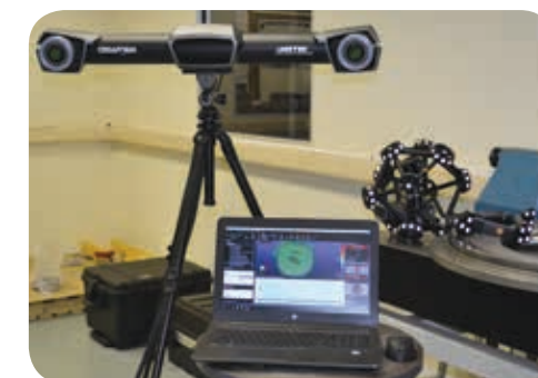
Accurate to within 30 µm, Necsa Nuclear Manufacturing's mobile laser-based scanning system can inspect a 4.0x4.0 m assembly from a single position while determining dimensional accuracy between multiple points selected using touch probes.
