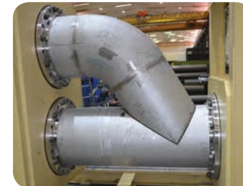
Following careful design of the SEC piping, welding jigs were manufactured for each individual section.
