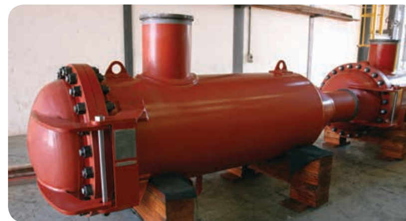
An intermediate strainer vessel manufactured by Necsa Nuclear Manufacturing according to the ASME VIII code for the ACCs of the Medupi power station.
