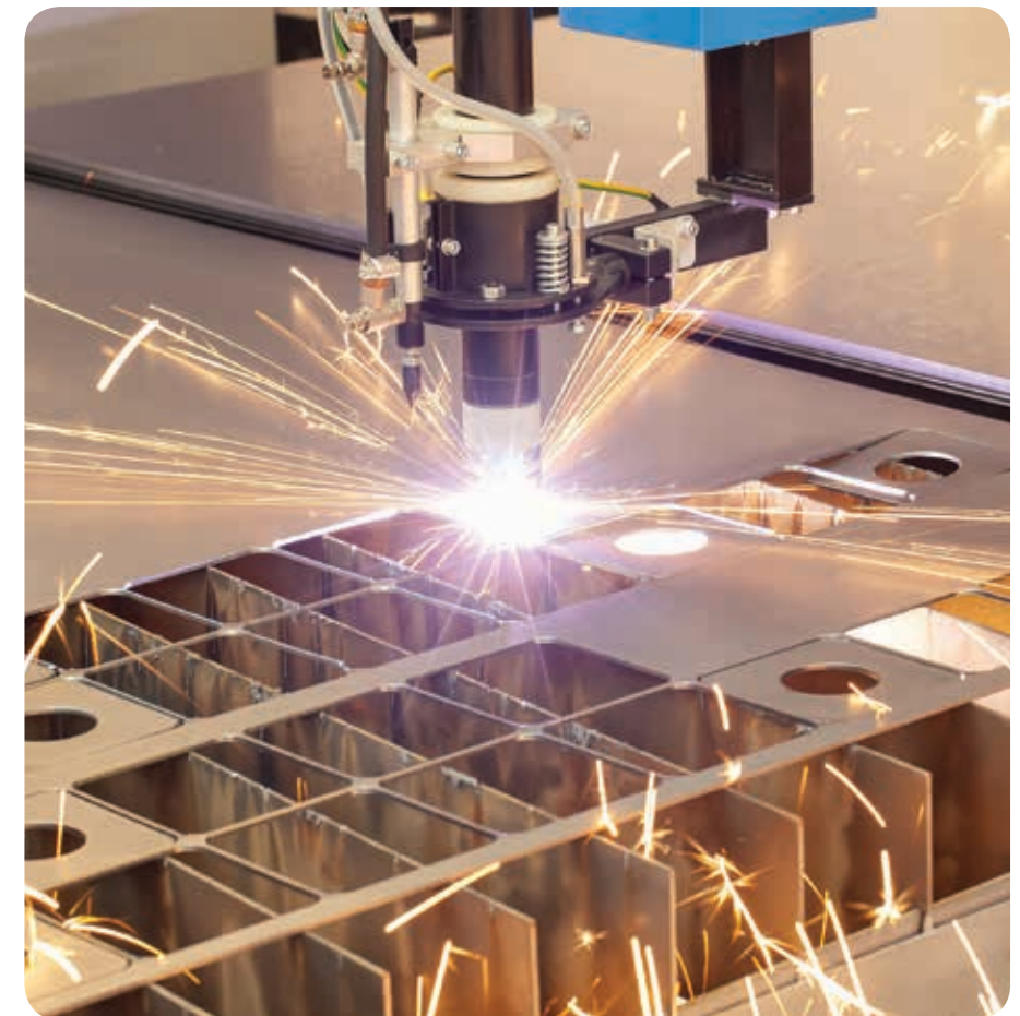
The plasma cutting process is restricted to cutting metals, including some of the reflective metals such as copper, brass and aluminium that cannot be cut with a laser. Material along the cut line is removed due to the very high temperature of the plasma arc and the high velocity of the gas jet generated by the constriction.
