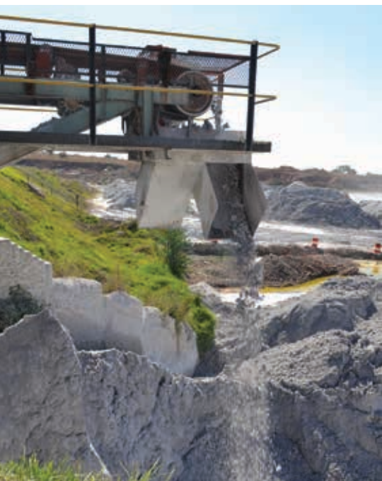
Product is transferred outside for sun and air drying down to 20% moisture required by cement plants.
