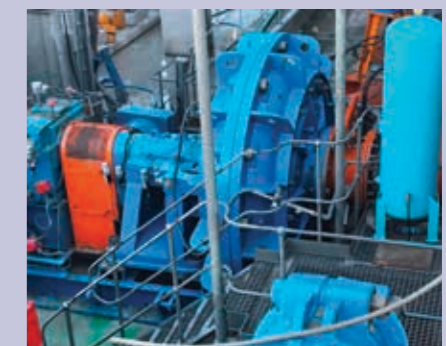
A Warman MCR 450 installed at Mogalakwena Mine. The MCR 450 runs at lower speeds resulting in lower wear rates on the parts.
