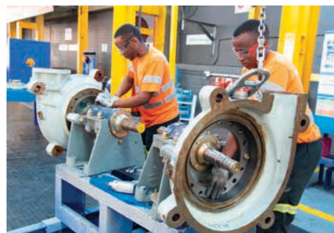
The local manufacturing process at Weir Minerals Africa includes foundry and assembly capacity for producing slurry pumps.
