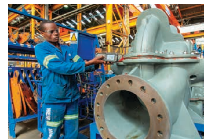
Pressure tests are conducted on slurry and dewatering pumps to ensure the quality of Weir Minerals' locally manufactured products.
