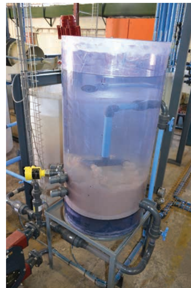
Volume flow and the rate of demineralisation can be varied by either increasing or decreasing the size or number of ion exchange tanks in each side of the battery.
