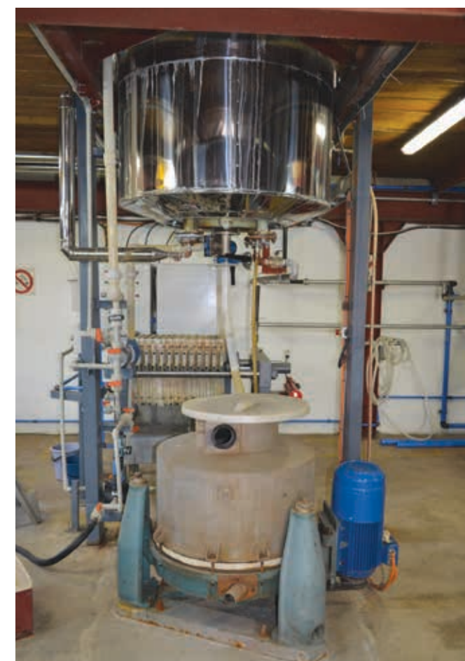
After precipitating out the multi charged cations, the residual sodium nitrate solution is mixed with an equimolar amount of potassium chloride and then evaporated. This causes the least soluble salt – sodium chloride – to crystallise out, leaving only the high-value potassium nitrate in the 'waste' cation regeneration solution.
