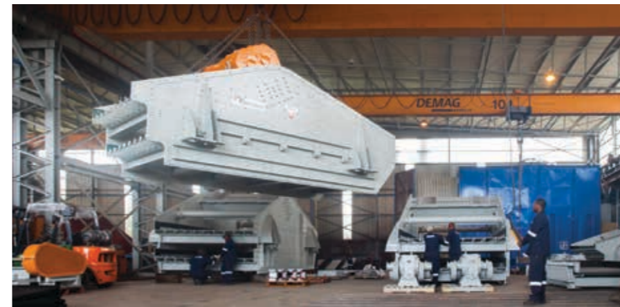
A Kwatani double deck screen order being finalised for dispatch on the shop floor.
