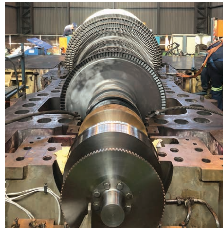
Marthinusen & Coutts took full responsibility for the entire drive train refurbishment on a 70 MVA generator set for the electrical generation plant at Metalloys' manganese plant in Meyerton, Gauteng.
