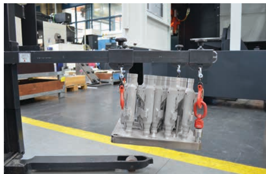
After 3-D printing, the base plates, together with the additively manufactured shafts, are transported to the bandsaw using an electric forklift truck.
