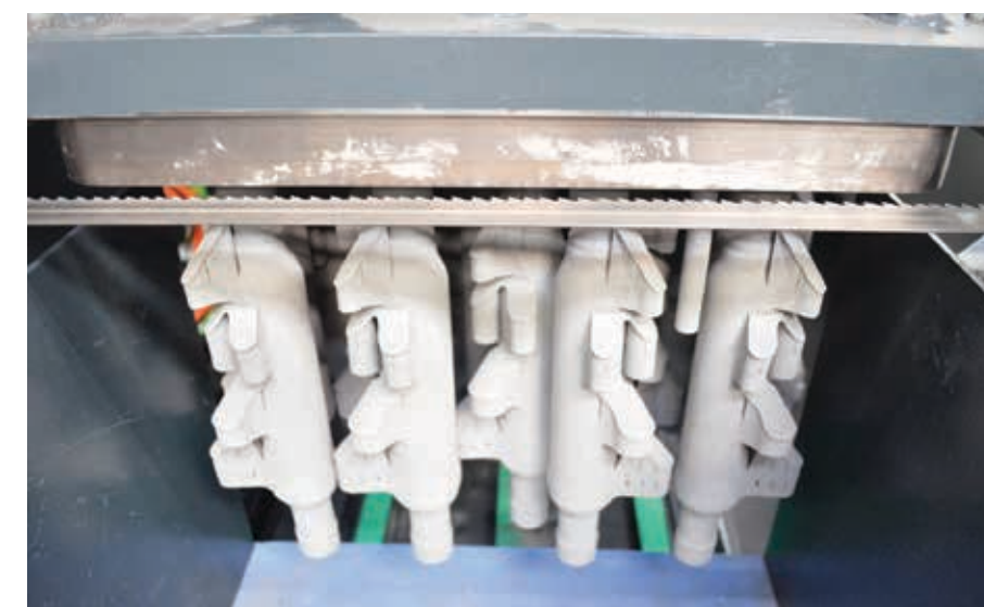
The operator measures the thickness of the clamped baseplate and enters its exact value using the AdvancedControl's job wizard. The top part of the saw, which is equipped with a high-precision ball screw spindle drive, then moves to the exact height required for cutting.
