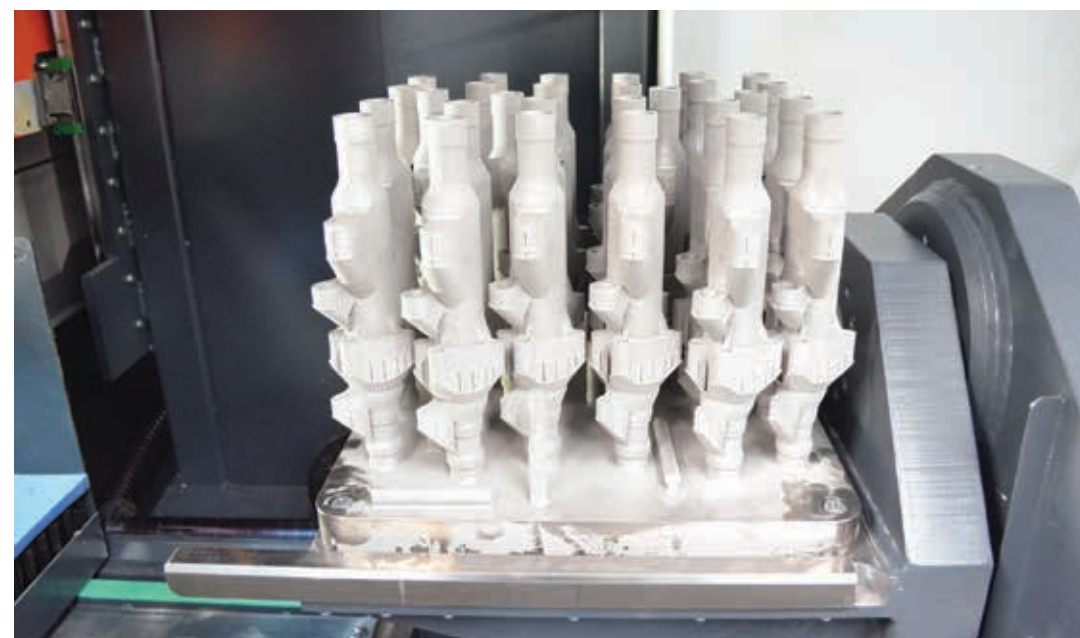
The titanium plates and components are then placed on the rotating clamping mechanism and attached using thick screws.
