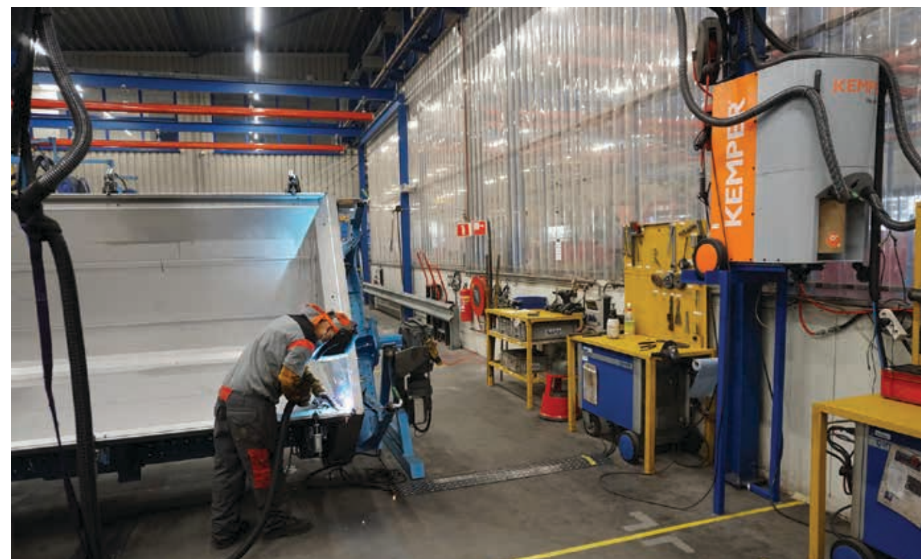
High-vacuum systems with connected extraction torches capture welding fumes directly at the point of origin while tracking of the source of fume as the welder moves the welding torch.
