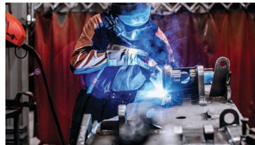
Above: Within the pulsed wire processes, Fronius has added PMC (pulse multi control), which offers a penetration stabiliser or an arc length stabiliser to make it easier for a manual welder to achieve the desired result.
