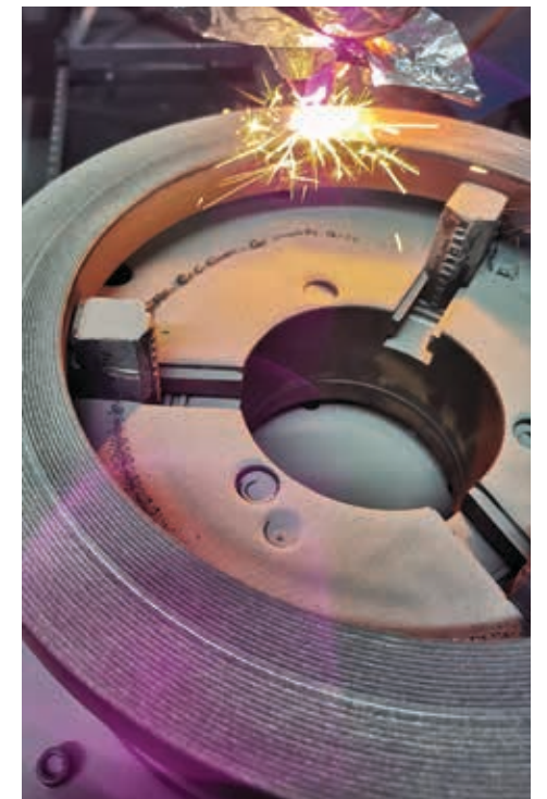
Laser cladding offers high levels of metallurgical flexibility, exceptionally low heat-input and dilution levels as low as 5.0%.
