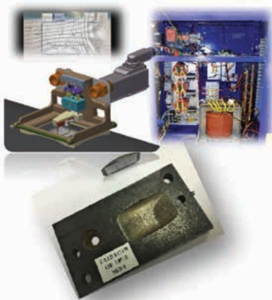
Figure 1: EDM Scoop Sampler with HMI and Control Trolley (Inset - EDM Scoop or 'boat' sample)
