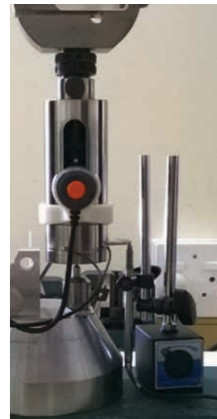
Figure 4: The SPT fixture, designed and fabricated by eNTSA for small disc testing.
