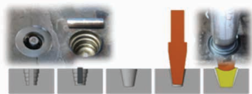
Figure 2: Schematic illustrating the WeldCore® process with photos of actual site procedure stages.
