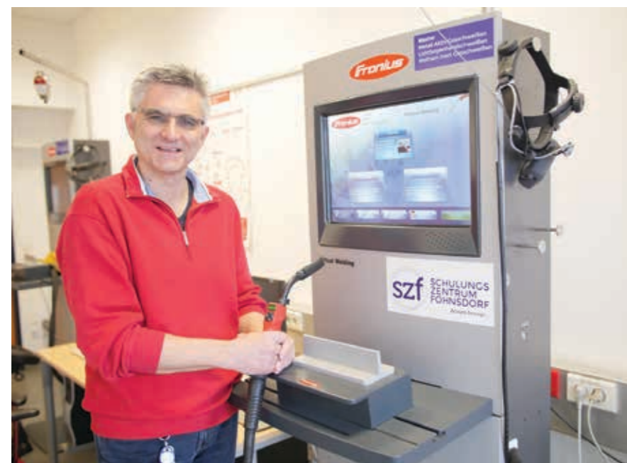
Hannes Krempl, welding technology and transport trainer at the Fohnsdorf Training Centre in Austria, reports that using the Fronius Virtual Welding simulator gives student welders 23% more practice time and reduces material costs by €230 per student.
