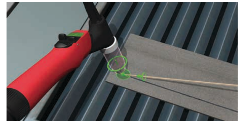
The Ghost is the virtual trainer that specifies the correct welding speed, the angle of the welding torch, and the torch to workpiece distance using visual guides (green in the image).
