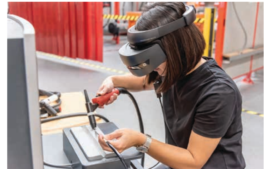
As with a flight simulator, 3D glasses provide particularly high resolution and sharpness, as well as a wide field of vision, resulting in a realistic welding experience.
