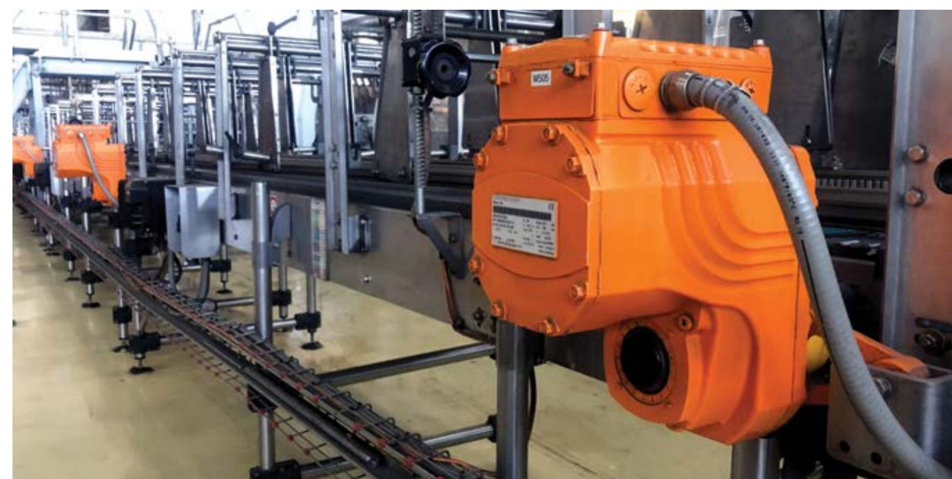
MOVIGEAR technology is ideal for conveying and packaging lines in the food and beverage industries, as well as a host of other light and dynamic production line applications.
