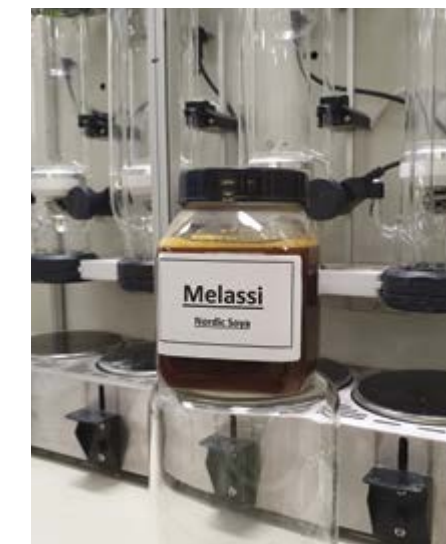
Soy molasses, which is unsuitable for food production, will be used as an alternative feedstock to sugar and corn in the manufacture of polylactic acid, (PLA). Photo: Nordic Soya.
