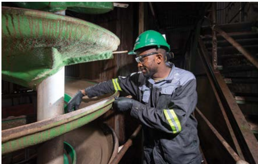
Multotec's new UX7 spiral for recovering ultra-fines has been tested on chrome, manganese and iron ore but can also be applied in the recovery of copper, platinum and other metals. Each application of the Multotec UX7 spiral will be based on an in-depth understanding of the customer's operating conditions.
