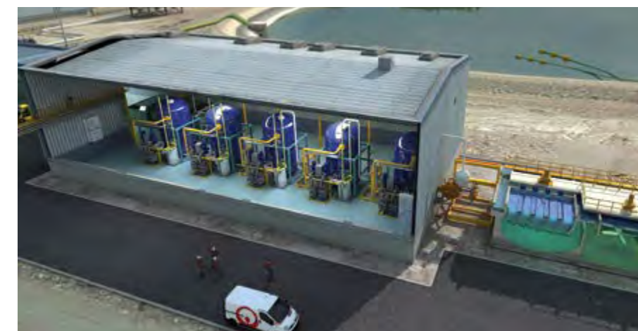
A Veolia filtration plant design for the front end of wastewater treatment, which comprises a settling plant followed by a Veolia Dual Media filtration plant.
