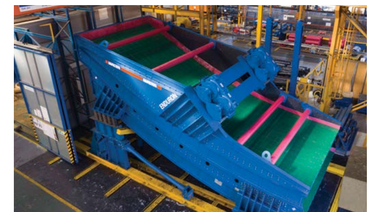
Two 51 t double deck Enduron DBHG 43/97 banana screens were designed from scratch, with the engineering team focusing on minimising mass without compromising structural integrity.
