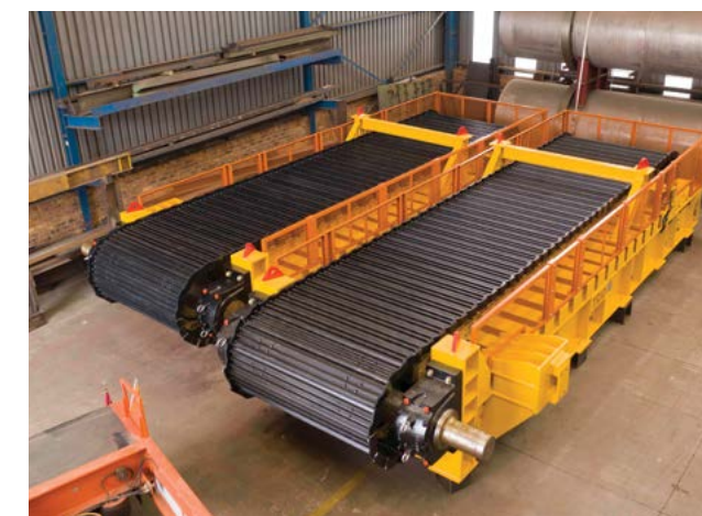
Two locally designed Trio apron feeders can each transfer 750 t/h of iron ore.
