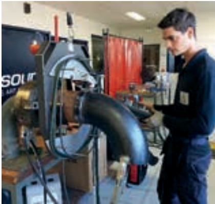
Orbital welding of a joint between a pipe and an elbow using an open orbital welding head of the MU family with arc voltage control and filler wire.
