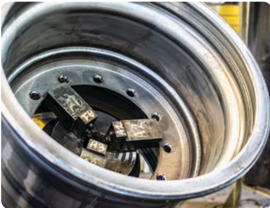
Above: Precise control of the welding process enables controlled droplet detachment and low heat input into the component, permitting low-spatter results with minimal distortion.
