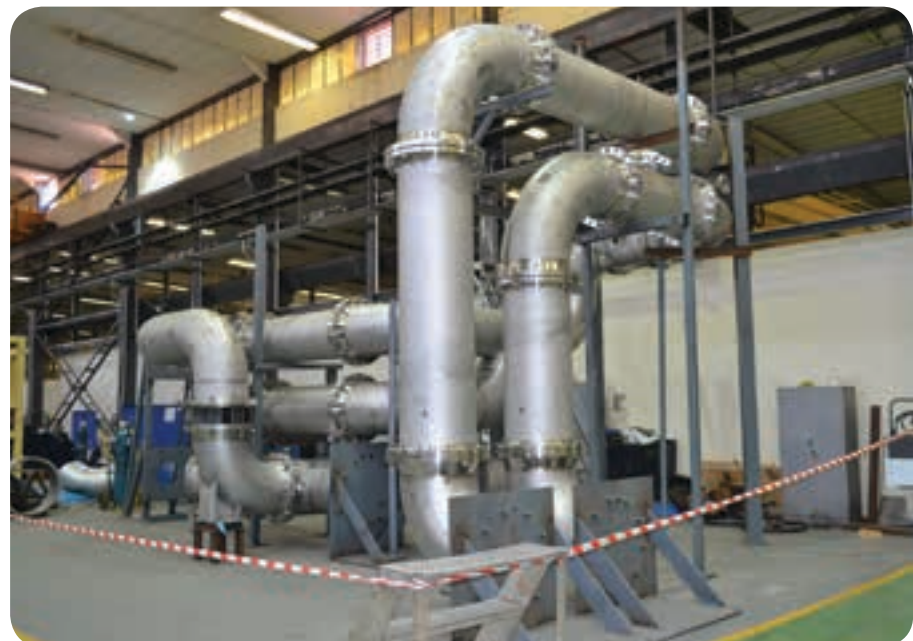
An assembly of SEC piping mocked up on Necsa Nuclear Manufacturing's shop floor to guarantee seamless installation onsite.
