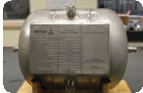
In January 2018, Nuclear Manufacturing supplied the first locally produced safety related ASME III designed and certified Air Receiver Pressure Vessel to Koeberg.
