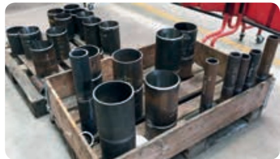
Pipe specimens prepared for the qualification of the orbital welding process by a certification body.
