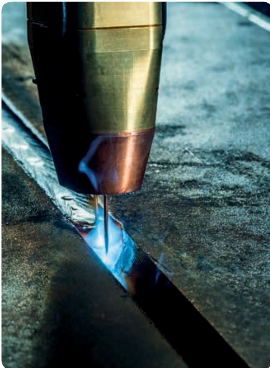
The tandem high performance welding process ensures that high-volume components and long seams are joined efficiently. The two wire electrodes are isolated from each other, allowing the arcs to be controlled individually.
