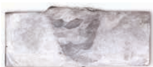
Above and right: Flaw-free macro and bend-test samples of the qualified test piece. “For the first time ever, we have a repeatable welding solution that offers high efficiency while maintaining weld quality,” says Conn Roux of Babcock.
