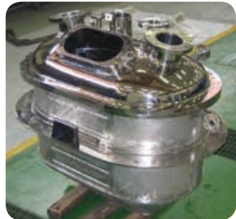
To avoid explosive reactions, vessels manufactured for Rheinmetall Denel Munitions in Potchefstroom had to be highly polished to avoid any substances get trapped in rough areas.
