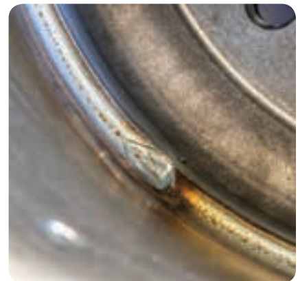
Above: Precise control of the welding process enables controlled droplet detachment and low heat input into the component, permitting low-spatter results with minimal distortion.
