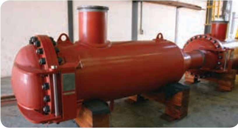
An intermediate strainer vessel manufactured by Necs Nuclear Manufacturing according to the ASME VIII code for the ACCs of the Medupi power station.
