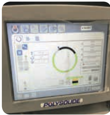
A real-time view of a welding cycle on the user Interface (GUI) of the Polysoude power source.
