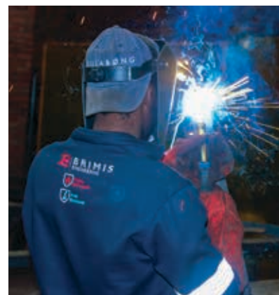
Brimis is moving towards the use of semi-automatic gas shielded metal arc welding (GMAW), especially for hardfacing using exotics such as Inconel 625 and Stellite.
