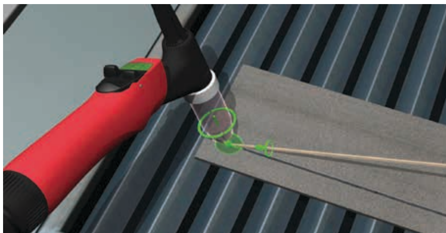
The Ghost is the virtual trainer that specifies the correct welding speed, the angle of the welding torch, and the torch to workpiece distance using visual guides (green in the image).
