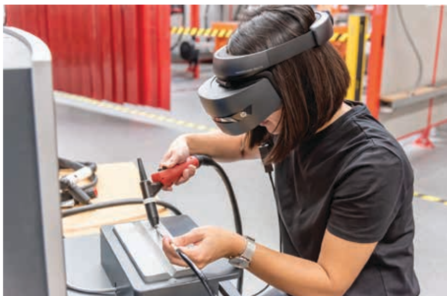
As with a flight simulator, 3D glasses provide particularly high resolution and sharpness, as well as a wide field of vision, resulting in a realistic welding experience.
