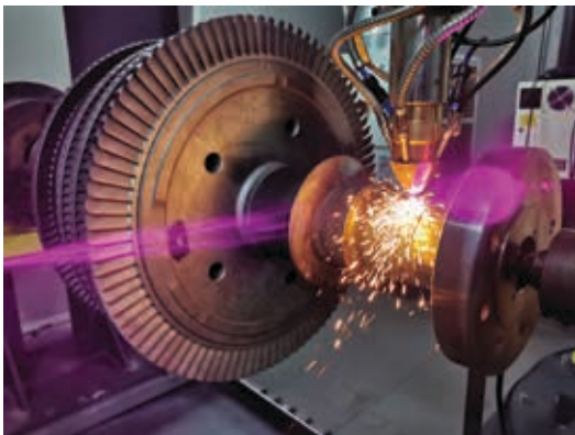
Laser cladding of a turbine rotor being done at Thermaspray's Olifantsfontein facility.
