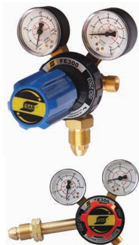
The recently launched ESAB GCE FE300 single-stage gas cylinder regulators fit into the medium- to high-tier product segment for use for oxy-acetylene or propane heating or cutting: Above: a 300 bar FE300 oxygen cylinder regulator. Red: a 40 bar acetylene cylinder regulator.
