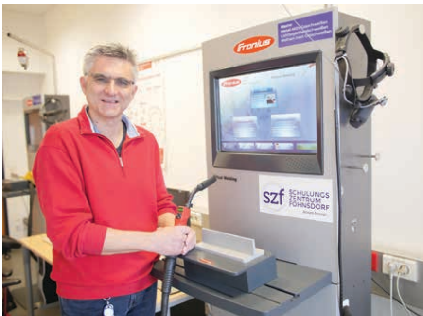
Hannes Krempel, welding technology and transport trainer at the Fohnsdorf Training Centre in Austria, reports that using the Fronius Virtual Welding simulator gives student welders 23% more practice time and reduces material costs by €230 per student.
