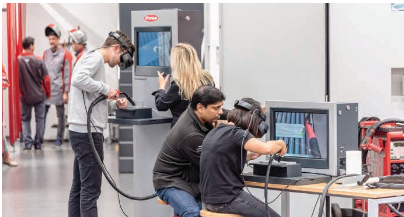
The Ghost is the virtual trainer that specifies the correct welding speed, the angle of the welding torch, and the torch to workpiece distance using visual guides (green in the image).
