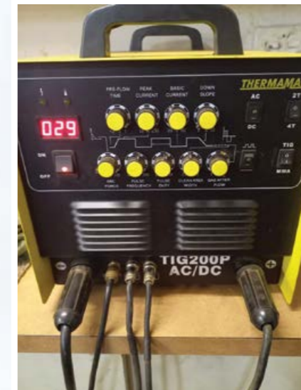
The Thermamax PRO-TIG 200 AC/DC welding inverter is a versatile machine that can accommodate aluminium and copper as well as mild and stainless steels.
