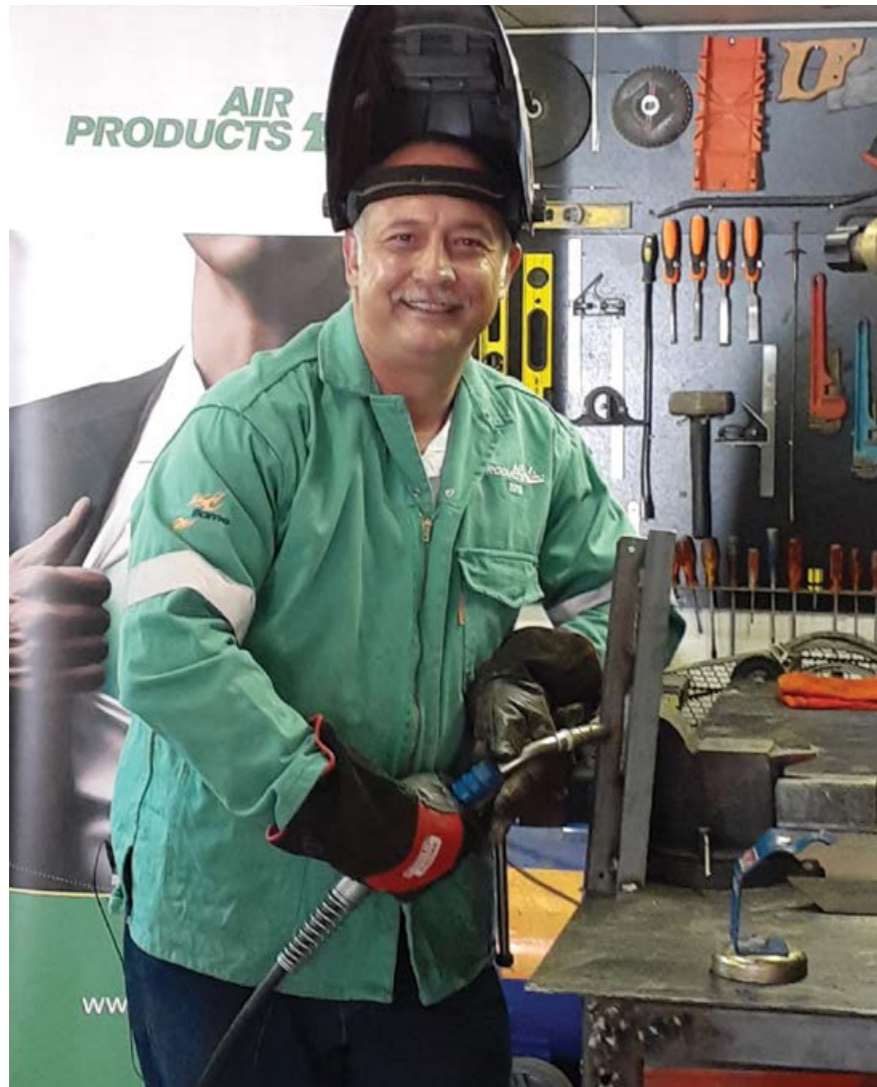
Air Products Welding Specialist, Sean Young, demonstrates the TIG/GTAW welding process.
