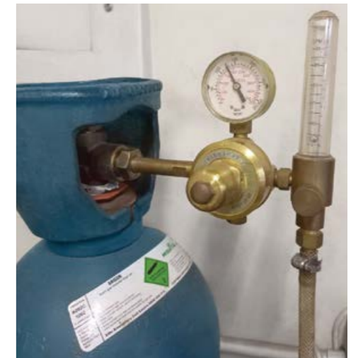
For TIG welding using a number six shroud a very low shielding gas flow rate of between 6.0 and 9.0 nine l/min is ideal shielding, says Young.
