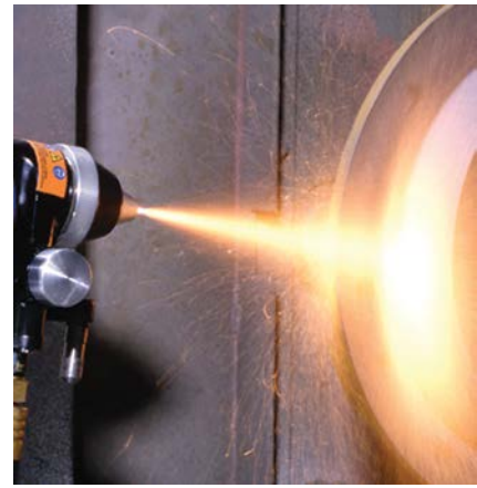
Wire flame spraying of steel.
