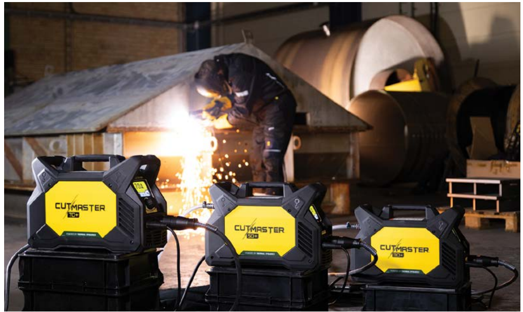
The Cutmaster+ family of handheld plasma cutting machines has a new TFT display and a large single button control knob. It comes with the SL60 1Torch, which features the 2T/4T function, a safety trigger lock, and double-tap trigger to conserve bottled air.
