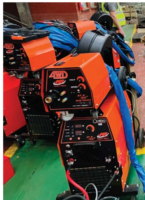
The Starweld CC/CV Quatro power sources delivered to Transnet. These machines are tunnel cooled to prevent contaminated cooling air passing over electrical and other components in the machine.
