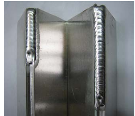
A 20 second aluminium TIG/GTAW welding comparison on thicker section plate using accurate at 150 A. Left: 100% Ar; Right, Ar+He.
