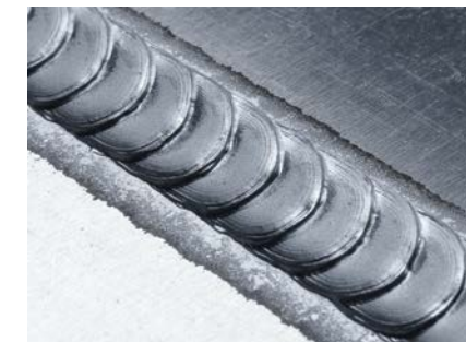
CMT Cycle Step enables welders to set both the number of individual droplets per welding spot and the pause time between cycles. This allows a high degree of precision and reproducibility, as well as a flawless weld seam.
