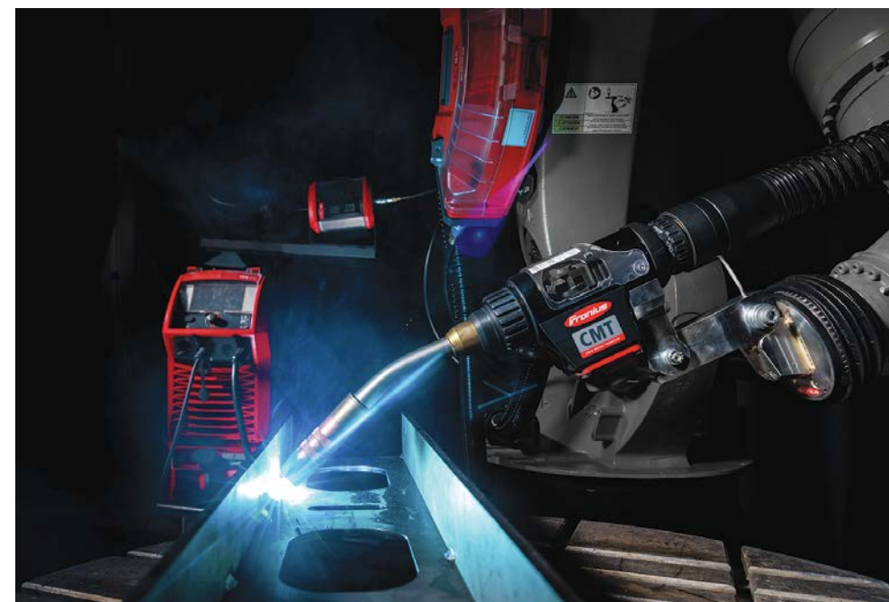
The highly dynamic and precise wire movement of the Robacta Drive CMT drive unit enables the reversing wire movement that makes CMT so unique.
