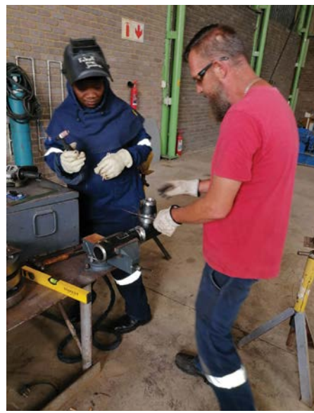
Left: Setting up a precision piping component and, right: the weldment prepared for TIG/GTAW welding.
