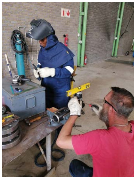
Left: Setting up a precision piping component and, right: the weldment prepared for TIG/GTAW welding.
