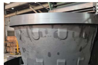
Machining a cast-iron component. AWT excels in repairing critical worn components with complex base materials and cladding surfaces using Stellite, Inconel, bronze, stainless steel and Monel.
