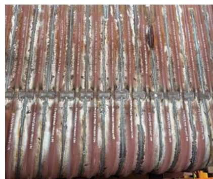
A boiler membrane wall panel. For long structural welds, Steinmüller uses a qualified metal-cored wire procedure. Laser cleaning is used before welding, and a weld prep primer is added after.
