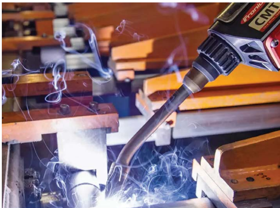
Fronius's modern CMT welding process can be tailored for surface engineering using many special alloys.
