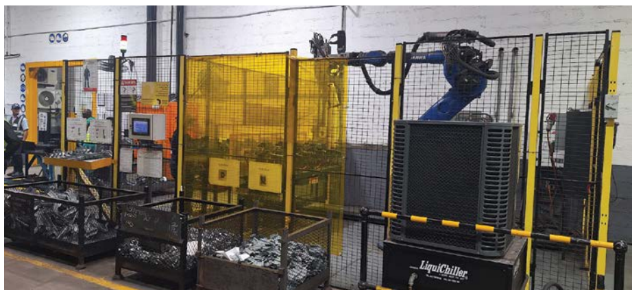
The latest collaboration project between D&L Engineering Solutions and Yaskawa Southern Africa is a component production line for the assembly of a safety critical automotive component.
