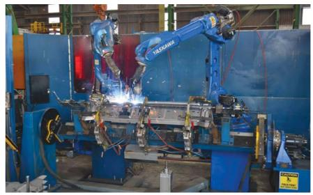
The safety-critical back panel for holding a vehicle's rear seatbelts is robotically-welded using advanced variable pulse MIG welding technology.
