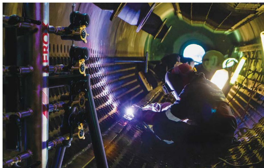
The Afrox multi-user pressure panel, or MUPP, has proved effective wherever several welders working in a confined space or at height need access to shielding gas.
