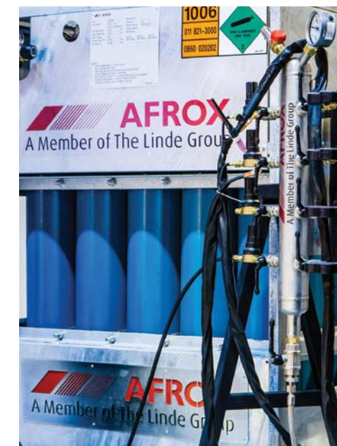
The shielding gas feeding each MUPP is supplied from manifolded cylinder pallets (MCP) of the specified shielding gas required, which are available in convenient bundles of 15 cylinders per pallet that can be managed from the ground.
