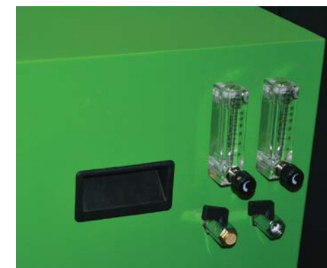
For shielding a laser weld, all that is needed is a gas flow of around 25 l/min, with the outlet pressure a little above atmospheric.
